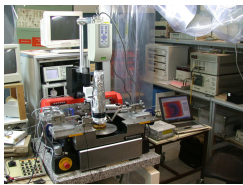
The Armines infrared bench could be fitted on the LAAS prober stations.
